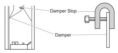
Figure 13 - Damper Stop Installation.
